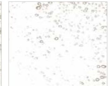
polyalphaolefin (PAO) air release: 12 seconds
